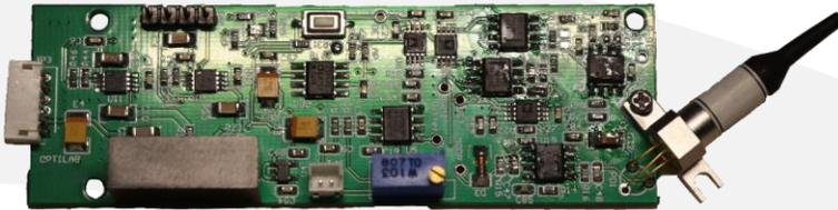
The Optilab BCB-4 is a compact bias control board designed for IMP-1064-20-PM modulator
