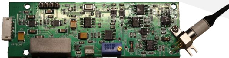
The Optilab BCB-4 is a compact automatic bias control board fully compatible with IMP-1064-40-PM modulator.
