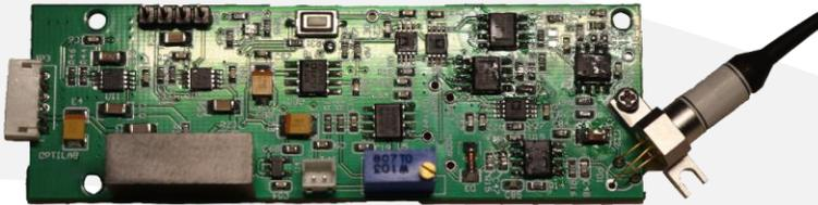
The Optilab BCB-4 is a compact bias control board designed for IMP-1064-10-PM modulator
