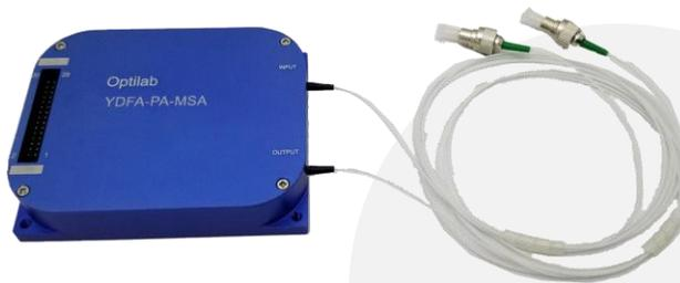
The Optilab YDFA-PA-MSA is a high-gain Dual Stage Pre-amplifier module in a multiple source agreement footprint housing.
