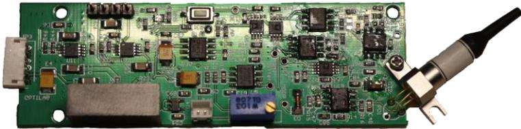
The Optilab BCB-4 is a compact bias control board designed to maintain the linear operating point of optical intensity modulators.
