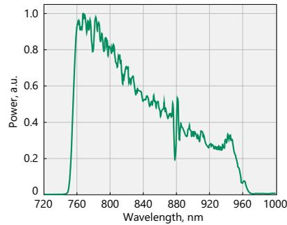
Fig 8. Typical output spectra of UltraFlux FF5010-F10 system
