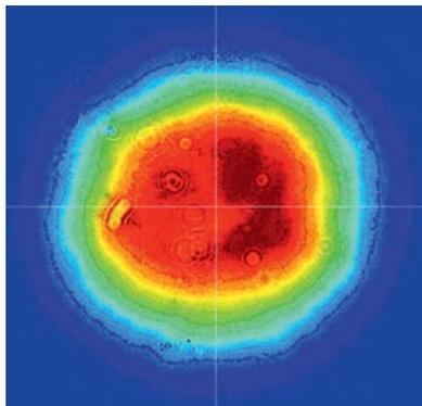
Fig 1. Typical UltraFlux FT310 near field beam profile
