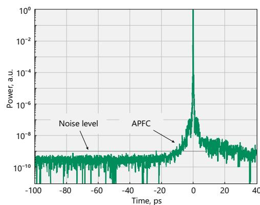
Fig 4. Typical temporal contrast of UltraFlux FF10010 system
