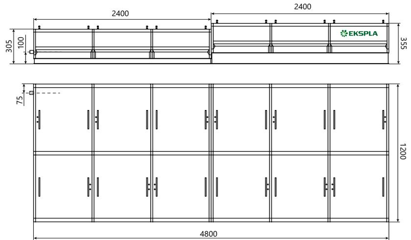
Fig 11. Typical UltraFlux FF5010-F10 laser system external dimensions
