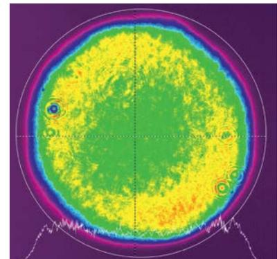
Fig 3. Typical UltraFlux FF8005 near field beam profile
