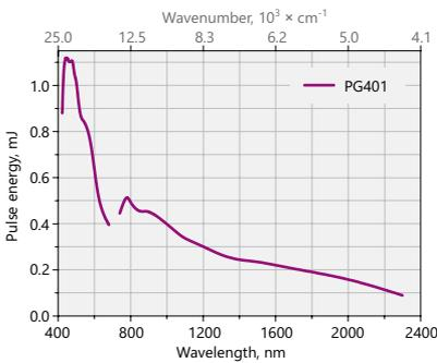
Fig 1. Typical PG401 model tuning curve
