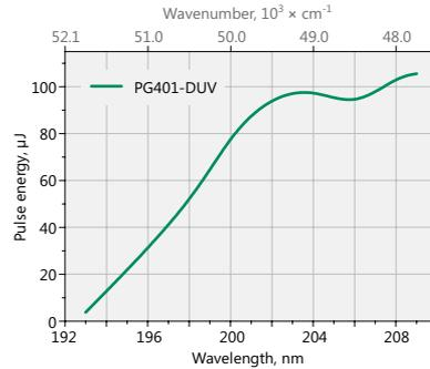
Fig 2. Typical PG401-DUV model tuning curve
