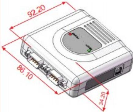
Dimensions are in millimeters
