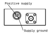
Supply connector (front view). The case is electrically connected to ground. There are two types of supply cable, one has 2 wires (new cable) and one has 5 wires (old). The corresponding color scheme of these cables is:
